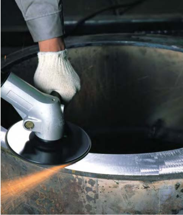
Model MAG-25B Depressed center wheel OD 58mm
