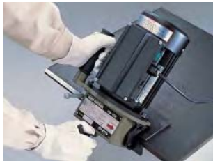
Beveling steel plates
