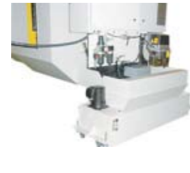
Coolant unit (tank)
