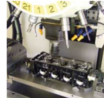
Four-face machining using an additional axis
