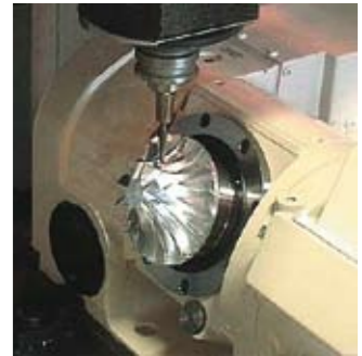
Three-dimensional contouring using two additional axes
