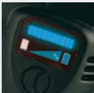
Battery condition display
