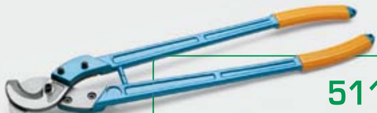
5116660500 For cutting cables 6 to 500 sqmm Weight: 3 kg Length: 800 mm
